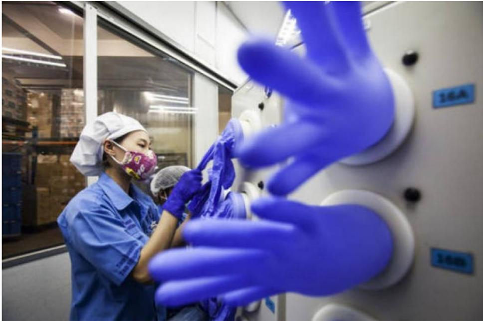
*Employees attach latex gloves to an air compressor as other gloves are inflated in the air-leak test room at a Top Glove Corp. factory in Setia Alam, Selangor. PHOTO: BLOOMBERG*
